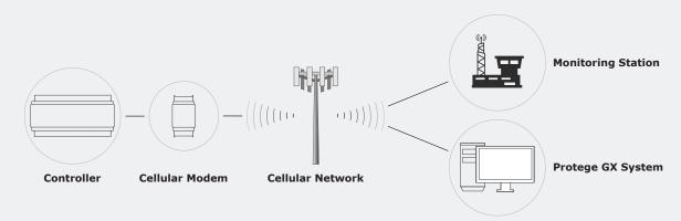
For Protege GX controllers the cellular modem also facilitates programming downloads and manual control from the Protege GX system, and event uploads to the Protege GX events database.
