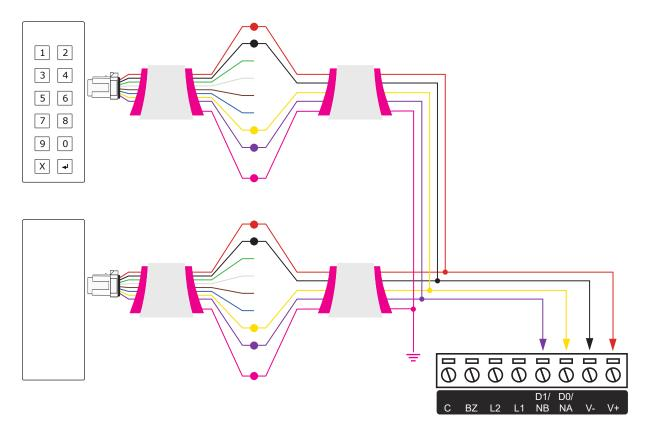
A 330 ohm EOL (End of Line) resistor may be required, inserted between the yellow and violet wires after the join.
