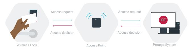
When a user presents their credential at a wireless lock operating in online mode the lock sends a request via the access point to check the credential's access permissions. The controller processes the request and provides an access decision. The lock grants or denies access accordingly, then sends the related events to the controller. When the user presents their credential at the next lock the process is repeated.
